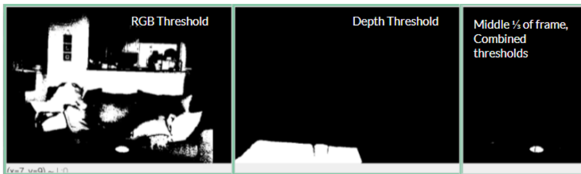
Figure 4. The leftmost image shows the RGB image with a threshold filter applied. The middle image shows the depth image with a threshold filter applied. The rightmost image shows the middle 33% of the frame, with RGB and depth thresholds overlapped.
